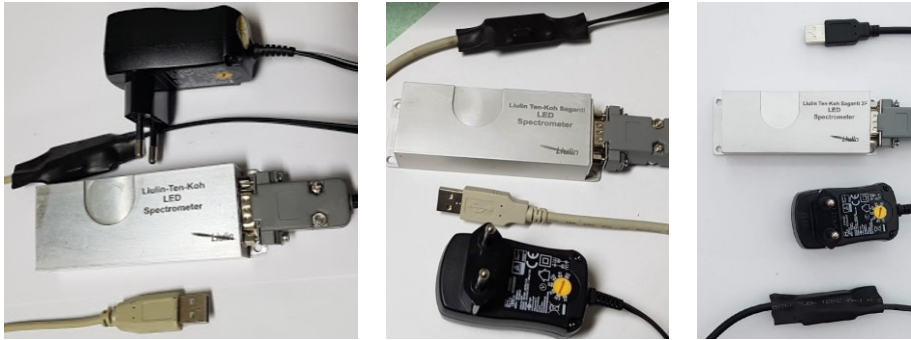
Fig. 1. External view of the 3 “Liulin Ten-Koh” instruments. The instruments are presented with the necessary: external power supply, RS-232 bridges and cables.
